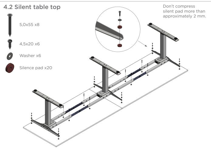
Loosen screws in crossbars and adjust stand width symmetric to desired position.
