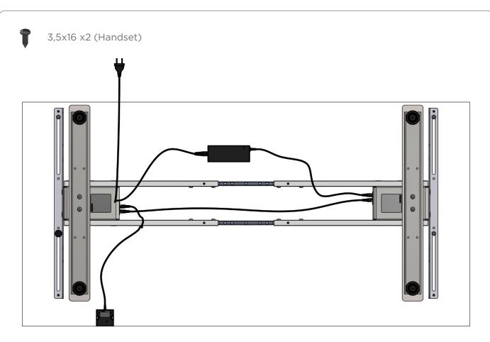
Structure excess cabling under the table top.
