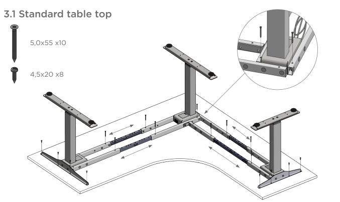
Loosen screws in crossbars and adjust stand width symmetric to desired position.
