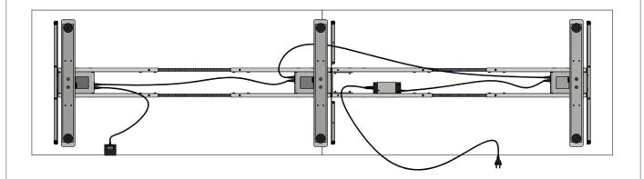
Structure excess cabling under the table top.
