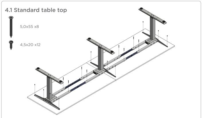
Loosen screws in crossbars and adjust stand width symmetric to desired position.
