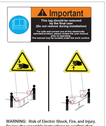
WARNING: Risk of Electric Shock, Fire, and Injury. Review the assembly instructions to confirm that the appropriate critical components and accessories are being used with the furnishing
