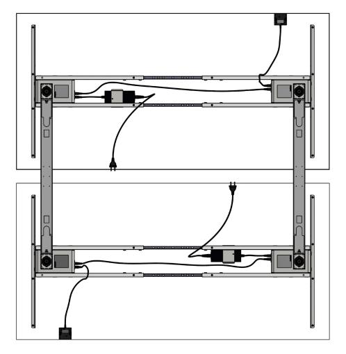
Structure excess cabling under the table top.
