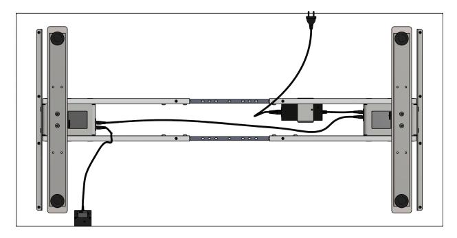
Structure excess cabling under the table top.
