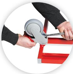
Tighten locknut with a 19 mm wrench.
