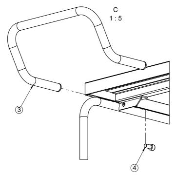
USE THE INCLUDED M10 HEX-KEY TO FASTEN THE HANDLE WITH M10-SCREWS.
