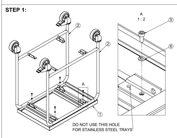
PUT ONE OF THE TRAYS UPSIDE DOWN ON A SOFT SURFACE AND PLACE THE FRAMES AS SHOWN IN THE PICTURE ABOVE.
